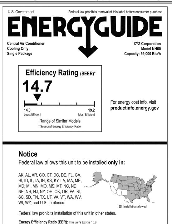
Sample Label 7B - Single-Package Central Air Conditioner (models manufactured after the compliance date of DOE regional efficiency standards in 10 CFR part 430)
