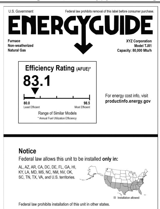
Sample Label 9 - Non-weatherized Gas Furnace (below 90 AFUE) (only for units manufactured on or after the compliance date of DOE regional efficiency standards in 10 CFR part 430)
