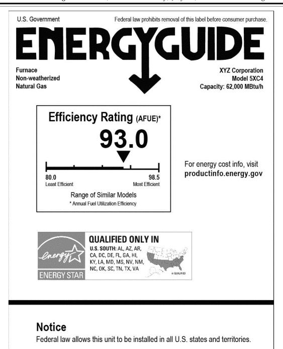
Sample Label 9A - Non-weatherized Gas Furnace (ENERGY STAR) (only for units manufactured on or after the compliance date of DOE regional efficiency standards in 10 CFR Part 430)
