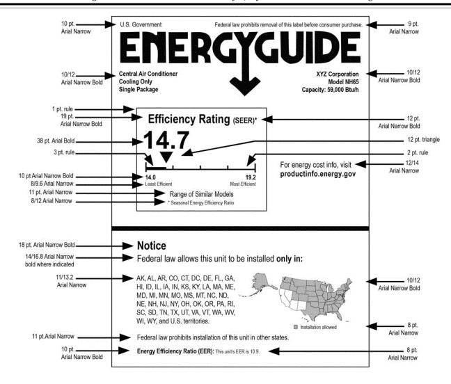
Prototype Label 3 - Single-Package Central Air Conditioner (models manufactured after the compliance date of DOE regional efficiency standards in 10 CFR part 430)
